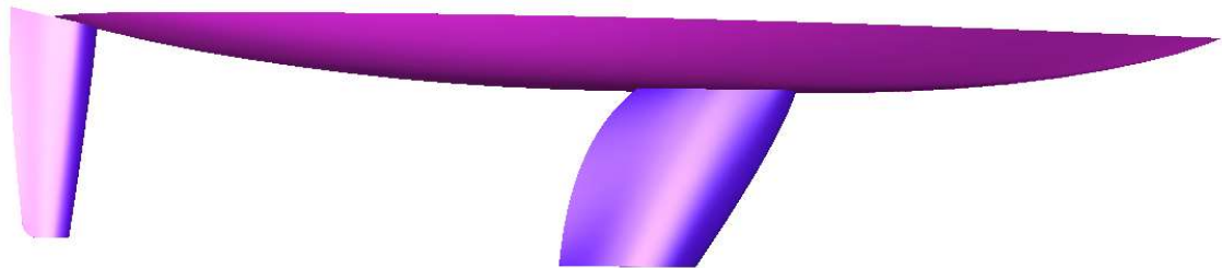
Fig 4-16(b) Arrangement Position of BBHH-Appendage under consideration stern form(about 0.321m forward) (in maxsurf)
