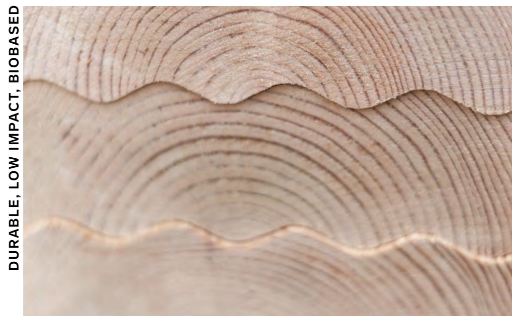
Wave-layered timber is a new innovation from the Finnish company Aalto Haitek. It creates extremely strong structures.
