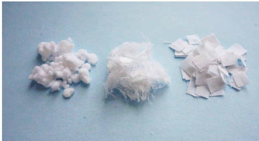
The recycling process OnceMore™ is turning worn out poly-cotton hospitable sheets into new textile fibre.
